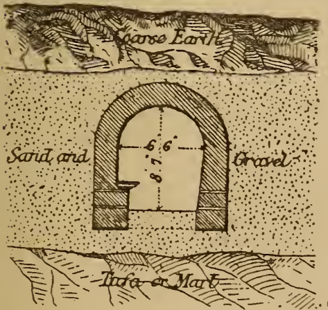
7316. Cross Section of New Gallery N o 4
